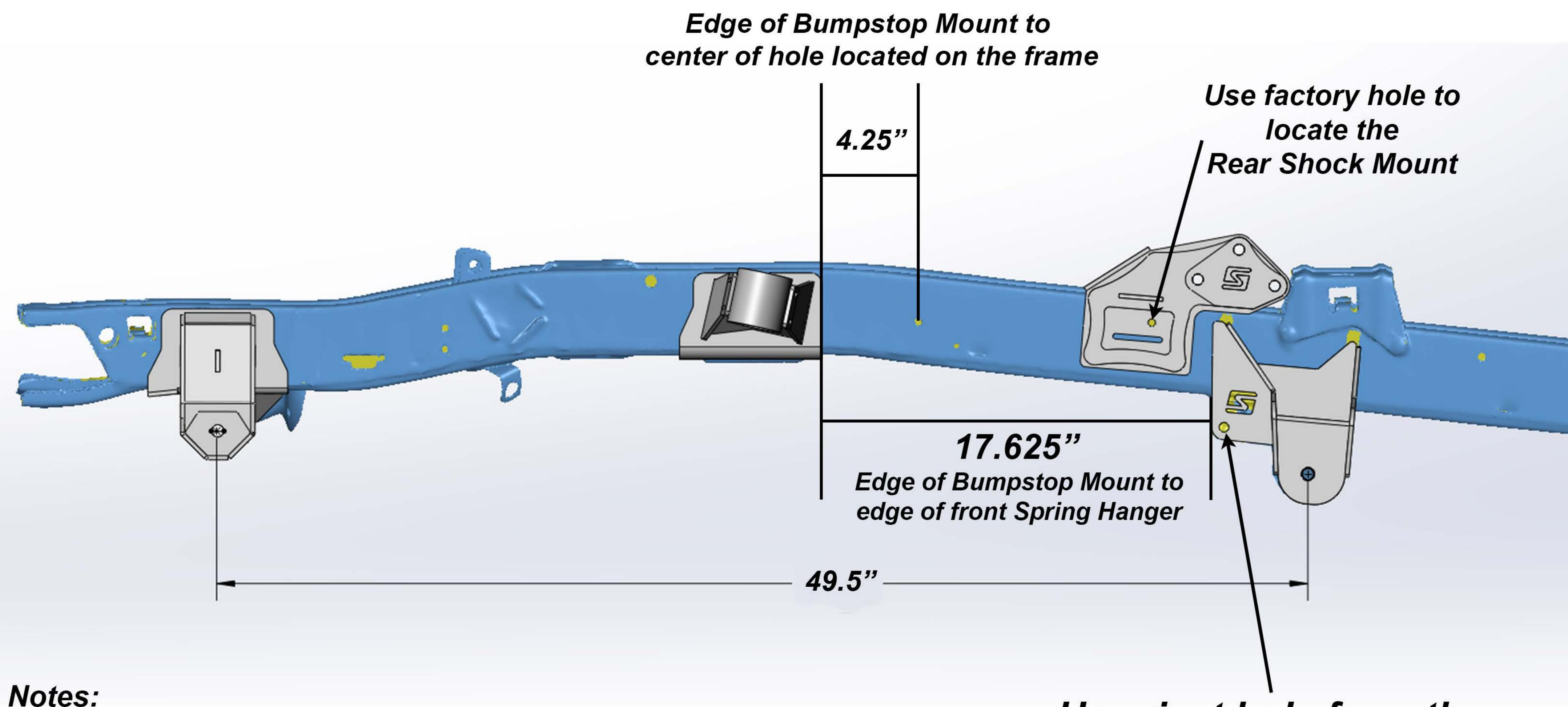
The factory Front Leaf Spring Hanger is two piece. Only remove the pice that holds the leaf spring. Leave the bottom factory "L" Bracket with the rivet holes.
